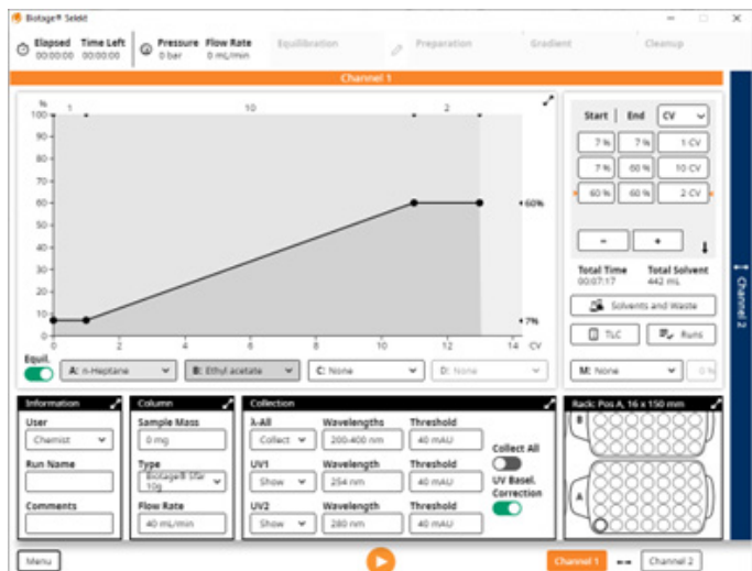
Figure 9. TLC-based linear gradient. The TLC strong solvent % was 30 which converts to a linear gradient of 7-60% over 10 column volumes (CV).
